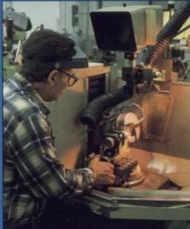
Exact geometries are ground on CBN tools with our sophisticated tool grinders.
