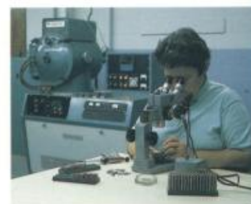
For phono points and stylii, we handset diamonds, then permanently bond them to steel in our specialized vacuum furnace.
