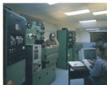
Precision cutting of polycrystalline diamond form tools, routers and grooving tools. Design engineers operate our CNC wire EDM systems.
