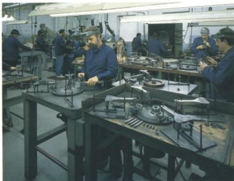
Skilled craftsmen grinding, lapping and polishing natural diamond tools.
