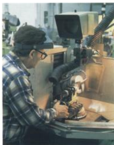
Exact geometries are ground on PCD tools with our sophisticated tool grinders.
